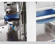
Quick disassembling belt for cleaning
